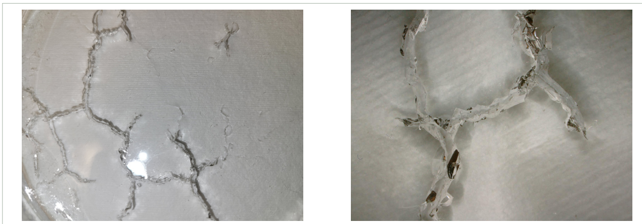
Figure 13a. Gel A surface condition, after 500 hours at -50°C
