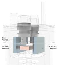
Double-opening contacts effectively double the opening distance based on the same motion of the moving contact bridge.
