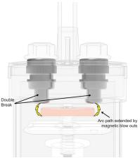
Magnetic blowouts effectively lengthen the opening distance by forcing the path of the arc to the outer edge of the contact chamber along magnetic field lines created by permanent magnets in the contact area. The magnetic field lines interact with the arc
