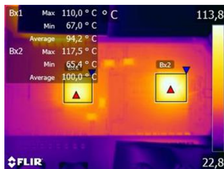
Figure 13. Temperature development during operation, forced-air cooling, 25°C ambient temperature
