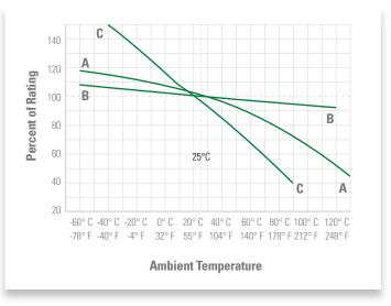
Curve A: Thin-Film Fuses and 313 Series (.010 to .150 A)
