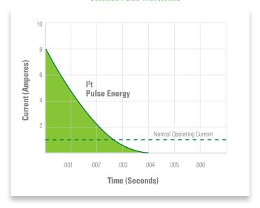
Step 2–Determine the required value of Nominal Melting I²t by referring to the Pulse Cycle Withstand Chart. A value of 22% is shown for 100,000 occurrences of the Pulse I²t calculated in Step 1. This Pulse I²t is converted to its required value of Nominal Melting I²t as follows:
