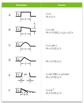
Step 3–Examine the l²t rating data for the PICO<sup>2®</sup>, 125 V, very fast-acting fuse. The part number 251001, 1-ampere design is rated at 0.256 A² Sec., which is the minimum fuse rating that will accommodate the 0.2327 A² Sec. value calculated in Step 2. This 1-ampere fuse will also accommodate the specified 0.75-ampere normal operating current, when a 25% derating factor is applied to the 1-ampere rating, as previously described.
