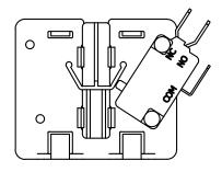
This Auxiliary Switch has a B600 rating. The B600 rating is defined by NEMA ICS 5: Industrial Control and Systems, Control Circuit and Pilot Devices standard.
