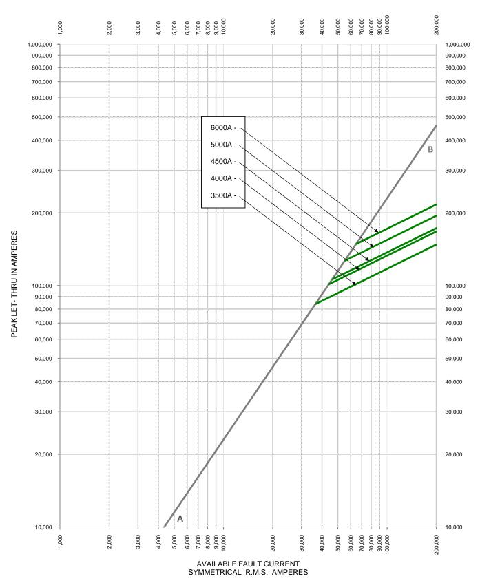
FUSE CATALOG NUMBER: TEST VOLTAGE: TIME CONSTANT/POWER FACTOR: KLPC 200A-6000A BASIS FOR DATA: AB = 15% Power Factor DRAWN BY: LLL LITTELFUSE, INC. CHICAGO, IL. USA DATE: 03/27/2018 REVISION: DRAWING NO.: SHEET 8 OF 9 PEAK LET-THRU CHARACTERISTIC CURVES
