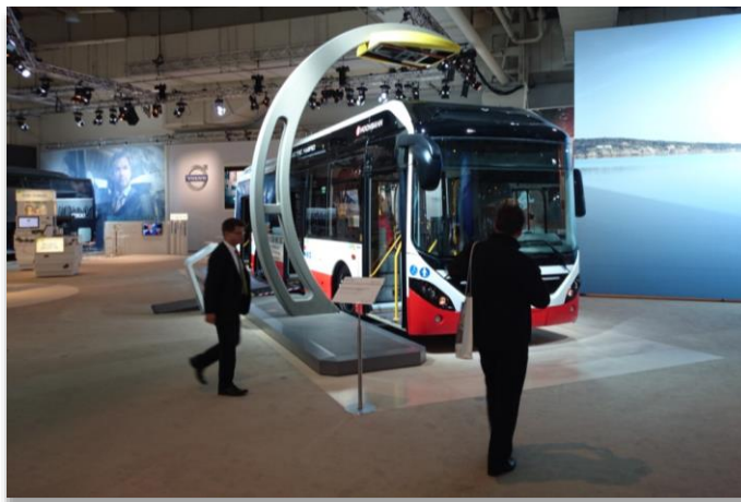
Figure 13. Top-down Pantograph for Opportunity Charging
