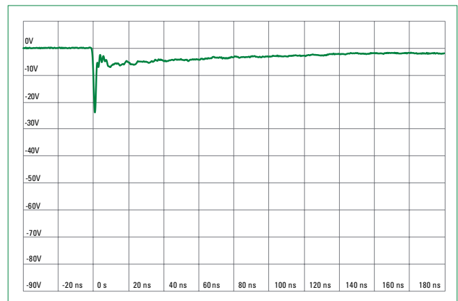
IEC 61000-4-2 -8 kV Contact ESD Clamping Voltage
