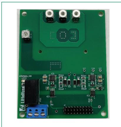
Figure 7. Top view of the test PCB having gate driver power supply, gate driver circuitry, and power connection terminal blocks
