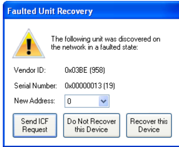
Figure 8 - Faulted Unit Recovery
