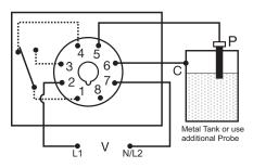
P = Probe C = Probe Common V = Voltage
