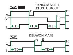
V = VoltageS1 = Initiate Switch L = Load (CR)E = Ready TD = Time Delay R = Reset
