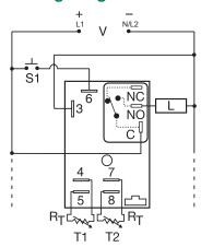
NO = Normally Open S1 = Reset Switch C = Common, Transfer Contact L = Load
