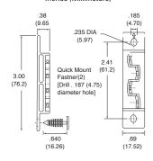
P0500-179 DIN RAIL MOUNT Inches (Millimeters)
