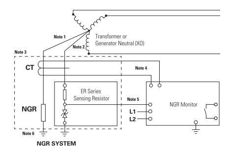
Note 1: Use minimum #8 AWG white or grey conductor insulated to system voltage to connect NGR to neutral.
