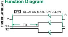
V = Voltage NO = Normally Open Contact NC = Normally **Closed Contact** TD = Time Delay R = Reset Time
