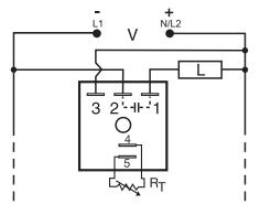
V = Voltage L = Load R<sub>T</sub> is used when external adjustment is ordered.
