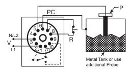
PC = Probe Common P = Probe V = Voltage R = Optional NC Reset Switch
