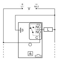
NO = Normally Open L = LoadC = Common, Transfer Contact
