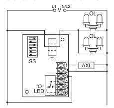
V = Voltage SS = Selector Switch T = Toroid AXL = Auxiliary Load/Alarm OL = Obstruction
