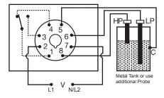
HP = HIGH LEVEL PROBE LP = LOW LEVEL PROBE C = PROBE COMMON V = VOLTAGE
