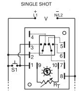
2-3 & 7-6 are Normally Open Contacts (NO) 2-4 & 7-5 are Normally Closed Contacts (NC)
