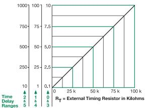
This chart applies to externally adjustable part numbers. The time delay is adjustable over the time delay range selected by varying the resistance across the R<sub>T</sub> terminals; as the resistance increases the tie delay increases
