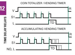
V = Voltage S1 = Initiate Switch NO = Normally Open Contact L = Load TD = Time Delay R = Reset
