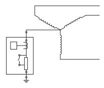
**Design Note 1:** An NGR conversion for a solidly grounded system requires a neutral connection to the existing power system, typically at the main transformer or switchgear. See *Figure 2*.
