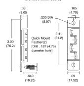
P0500-179 DIN RAIL MOUNT Inches (Millimeters)
