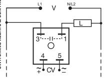
V = Voltage CV = Control Voltage L = Load
