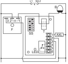
V = Voltage B = Beacon Lamps SS = Selector Switch T = Toroid F = Flasher AXL = Auxiliary Load/Alarm
