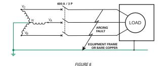
Assume that this ground-fault is not a bolted fault, but an arcing fault due to an insulation breakdown or a partial reduction of clearances between the line and ground.
