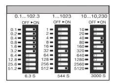
\*For CE approved applications, power must be removed from the unit when a switch position is changed.
