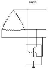
**Design Note 1:** A zigzag conversion requires a three-phase connection to the existing power system, typically at the main transformer or switchgear. See *Figure 1*.
