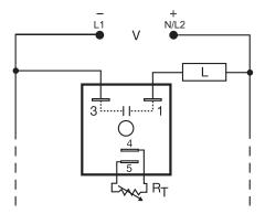
Load may be connected to terminal 3 or 1.
