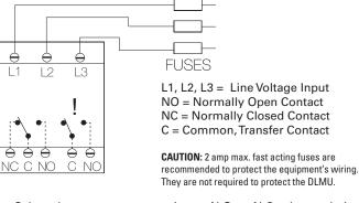
! = Select alarm contact connection as N.O. or N.C. when ordering; N.O. Shown.
