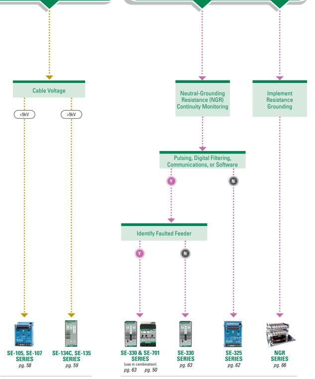
Ground-Conductor Monitoring Relays
