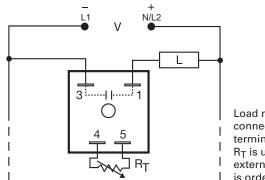
Load may be connected to terminal 3 or 1. R<sub>T</sub> is used when external adjustment is ordered.
