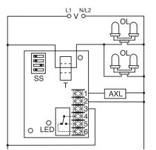
V = Voltage OL = Obstruction Lamps T = ToroidSS = Selector Switch AXL = Auxiliary
