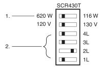
Example Shown: SCR430T-620 watts at 120 VAC lamps, two lamps are ON during normal operation.
