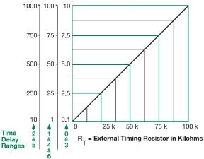
This chart applies to externally adjustable part numbers. The time delay is adjustable over the time delay range selected by varying the resistance across the RT terminals; as the resistance increases the
