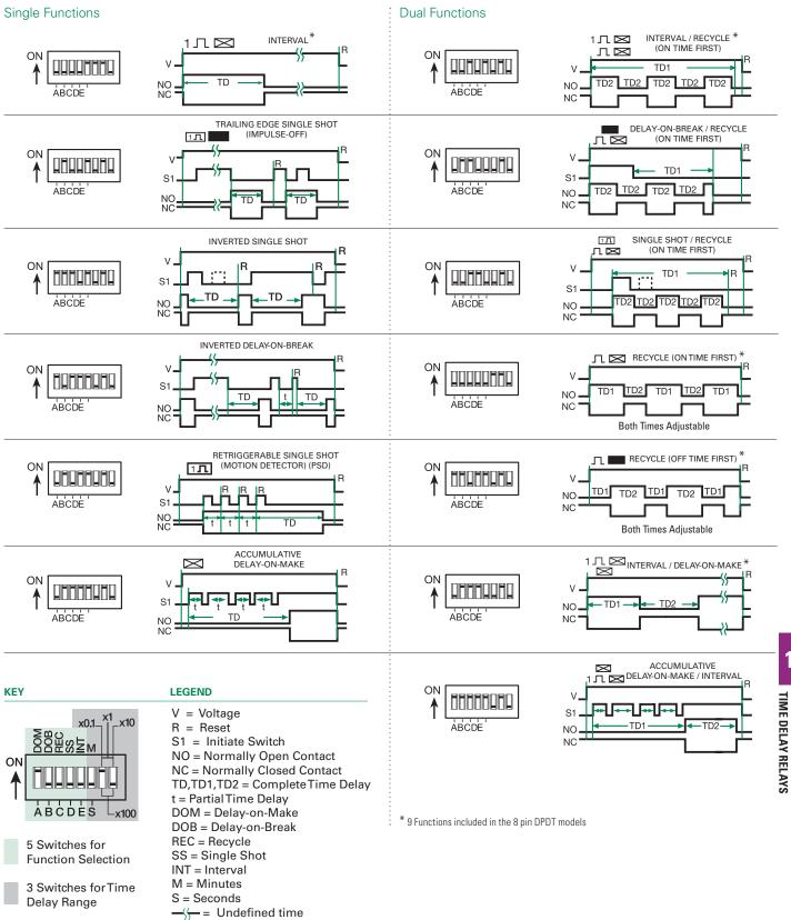
NOTE: The time delay range is the same for both functions when dual functions are selected.
