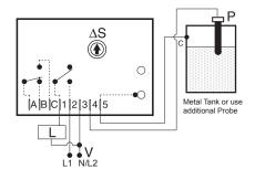
P = Probe L = Load V = Voltage ΔS = Sensitivity Adjustment
