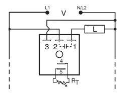
R<sub>T</sub> is used when external adjustment is ordered.
