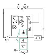
V = Voltage S1 = Initiate Switch C = Common, Transfer Contact UTL = Untimed Load (optional)
