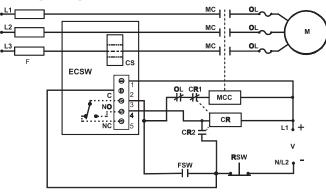
MC = Motor Contactor M = Motor F = Fuses OL = Overload RSW = Reset Switch FSW = Fan or Float Contacts CR = Control Relay CS = Current Sensor MCC = Motor Contactor Coil
