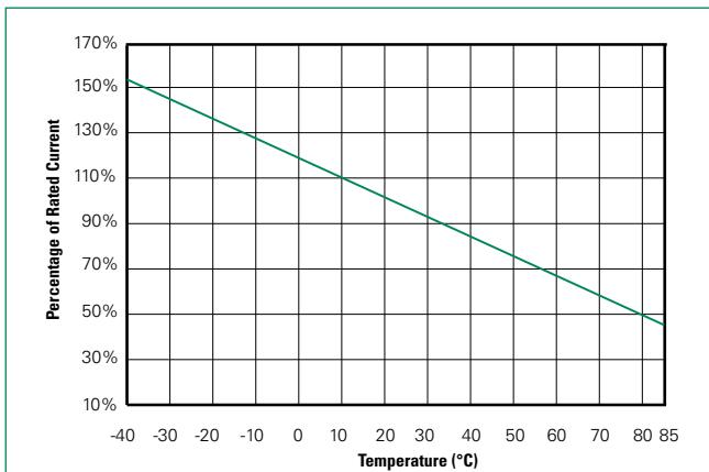
**Note:** Typical Temperature rerating curve, refer to table for derating data
