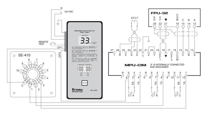
Let us consider an FPU-32 providing overcurrent protection according to an IEEE Very Inverse time-current curve. We will assume that 1200 A of current is flowing through the window of one of the 800:5 phase current transformers. We will also assume an FPU-32 inverse-time-overcurrent pickup setting ( $I_p$ ) of 1.0.
