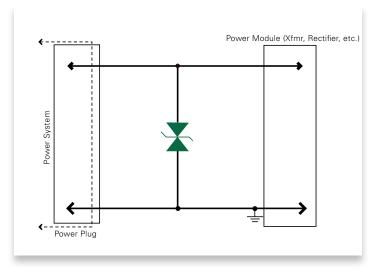
Using high-power TVS Diodes in a power supply configuration offer advantages over conventional methods, including no wear-out mechanism, faster response, and compact design.
